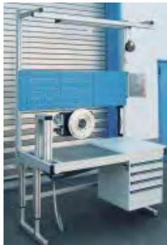
Assembly service table with lockable rotating unit for vacuum pumps
