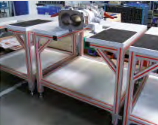
Assembly line for pumps of profile Series 50 with closed profile T-slots via closure strip, red
