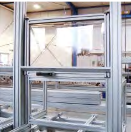
Manual vertical door equipped with counter balances inside profile, attachment with cable and pulleys and optional weight adjustment
