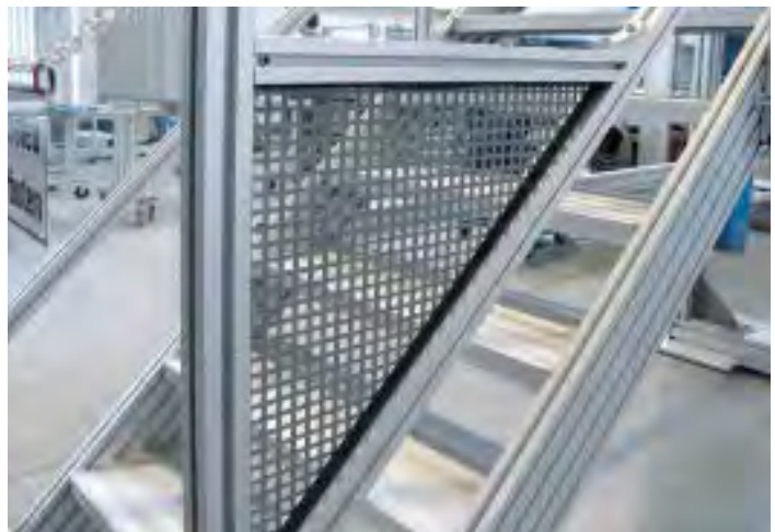
Tread with perforated plate for signs or warnings
