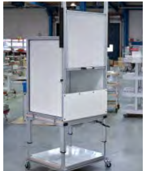
Workstation with protective fluid and manually adjustable sliding element
