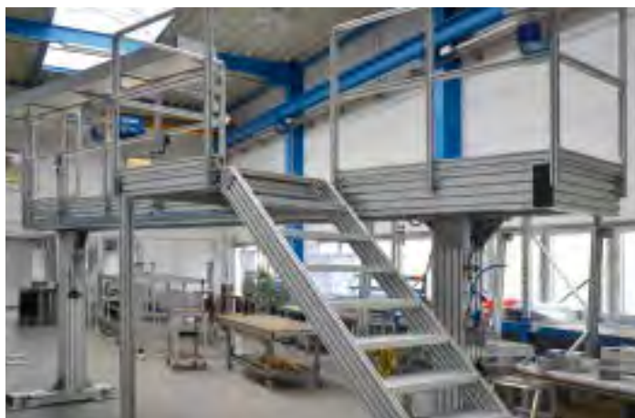
Self-supporting assembly platform with 45° stairs
