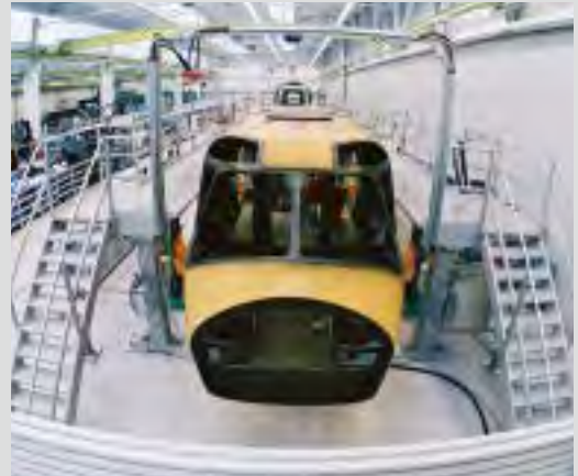
Platform for easy and safe maintenance and assembly work on helicopters
