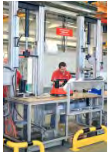
Assembly workstation with integrated press and document tray
