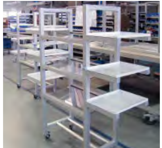
Material supply trolleys made of clean room Series 40 profiles incl. acrylic shelves
