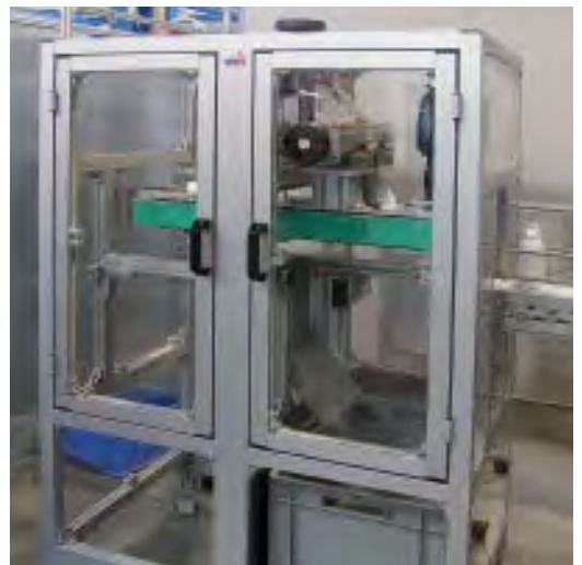
Guarding with swing doors made of clean room profiles
