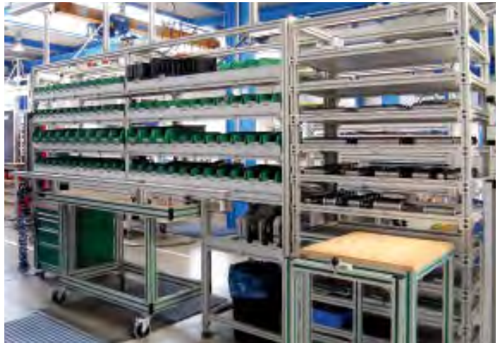
Workstation following the "Kanban principle" for productivity-enhancing decoupling of assembly and supply logistics
