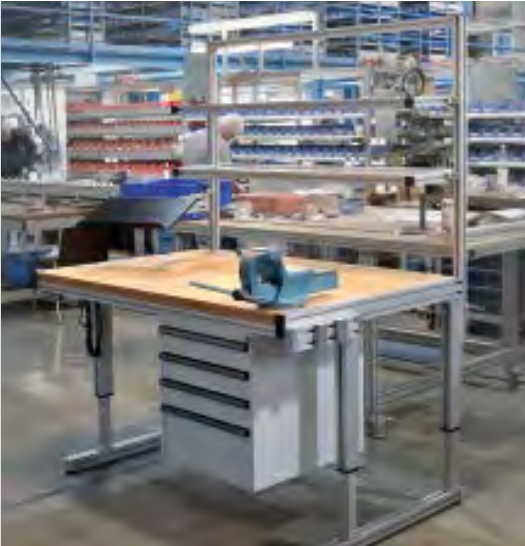
Workstation with electro-hydraulic height adjustment and hanging cabinet
