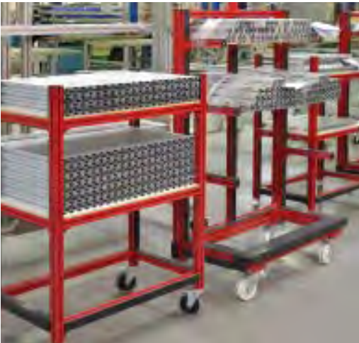
Supply trolleys made of Series 40 profiles, painted red
