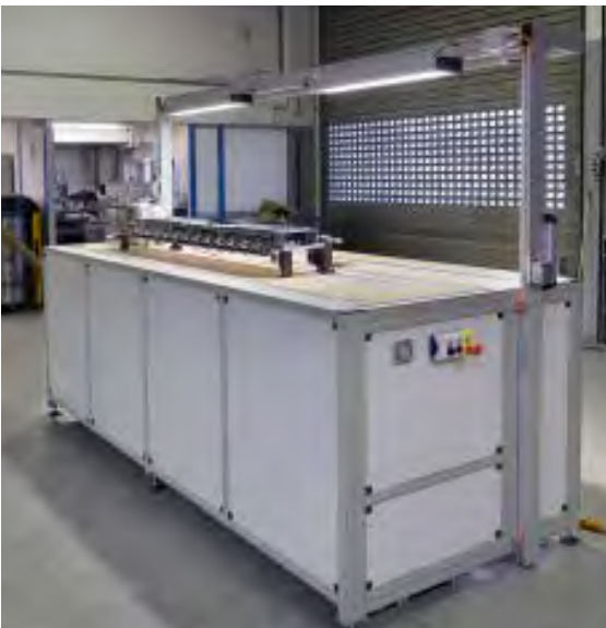
Assembly workspace with lowering device for electrically powered hydraulic cylinders
