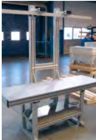
Assembly workstation using a crank for manually adjustable heights, load capacity 600 kg
