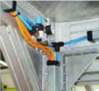
Empty grooves offer multiple options to route electrical supply lines
