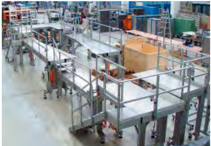
Cantilever assembly platform, 15 meter, with load steps for secure grip for heavy loads
