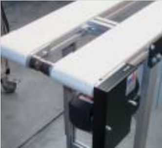
Two conveyor belts driven by one motor at the head drive
