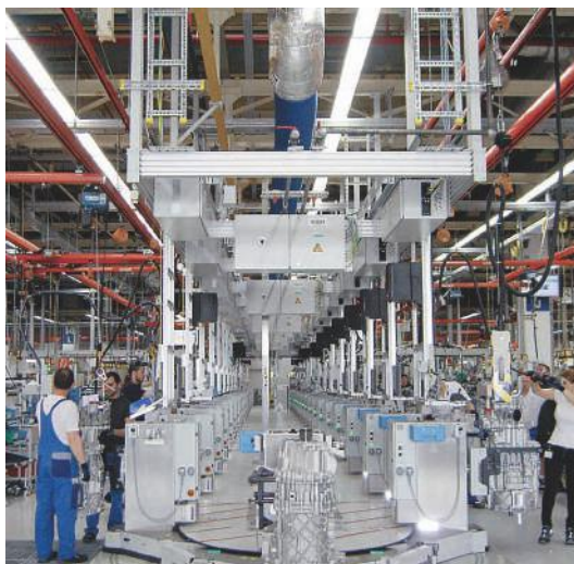
Overhead structure built from Series 40 profiles to support supply lines for assembly workstations
