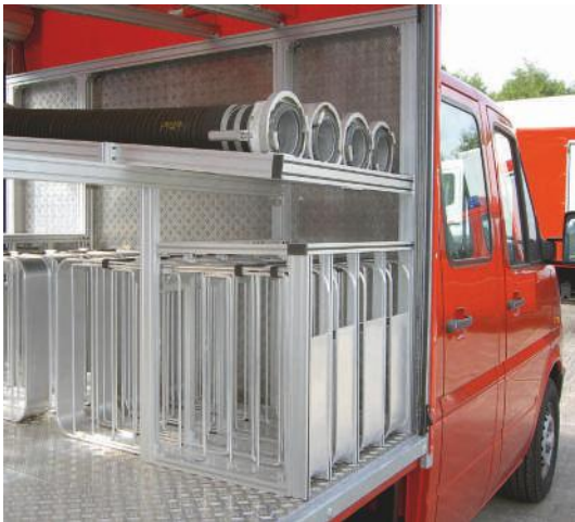
Fire engine interior built from Series 25 profiles
