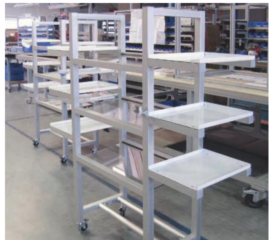
Material supply trolleys made from Series 40 cleanroom profiles with acrylic shelves
