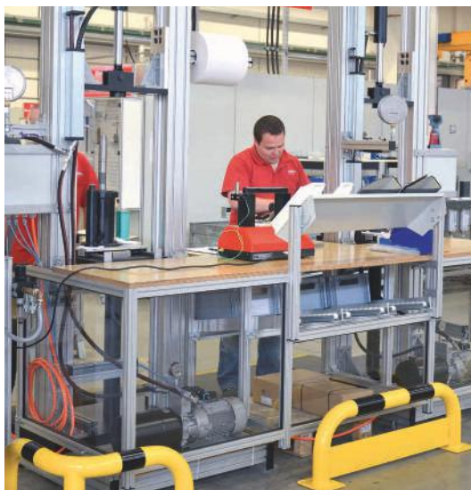
Assembly workstation with integrated press and document holder
