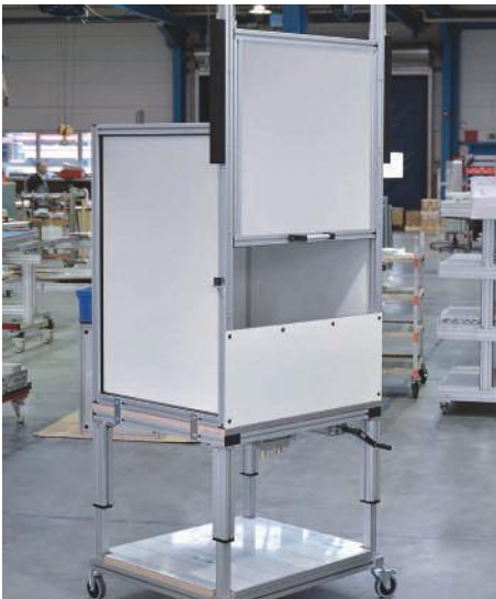
Workstation with protective cover and manually adjustable sliding element
