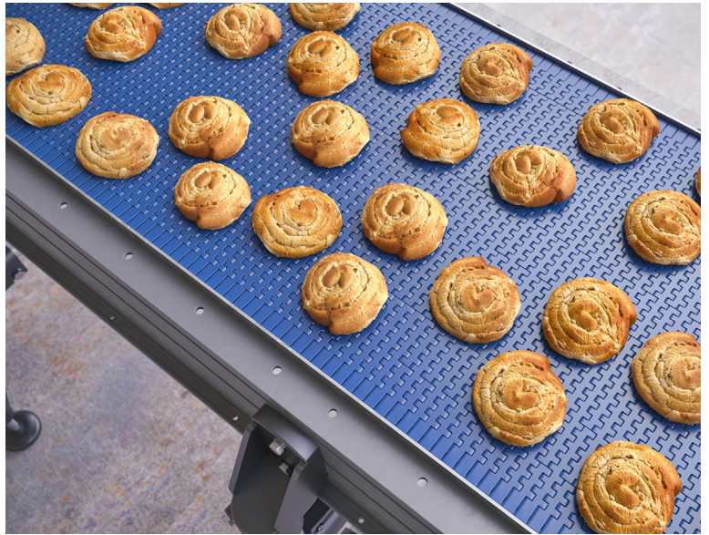
Conveyor equipped with Rexnord 595 Series KleanTop Belt.
