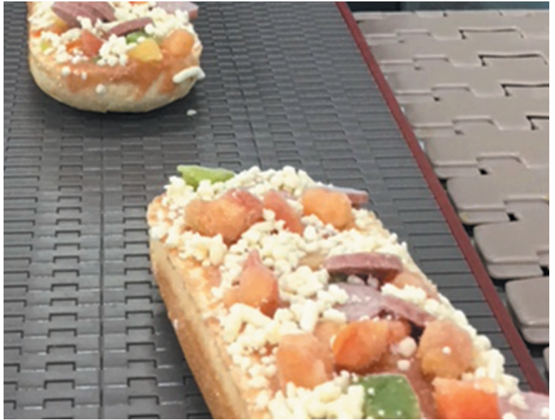
Conveyor equipped with Rexnord 395 Series KleanTop Belt.
