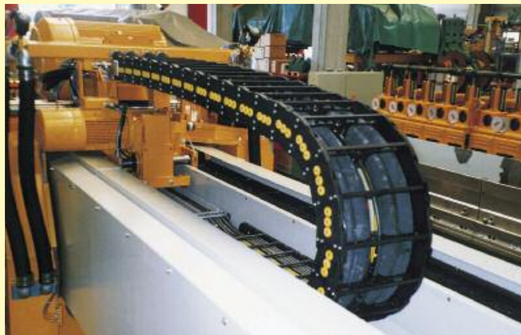
Nylon chain, type 310, in a self-supporting state.
