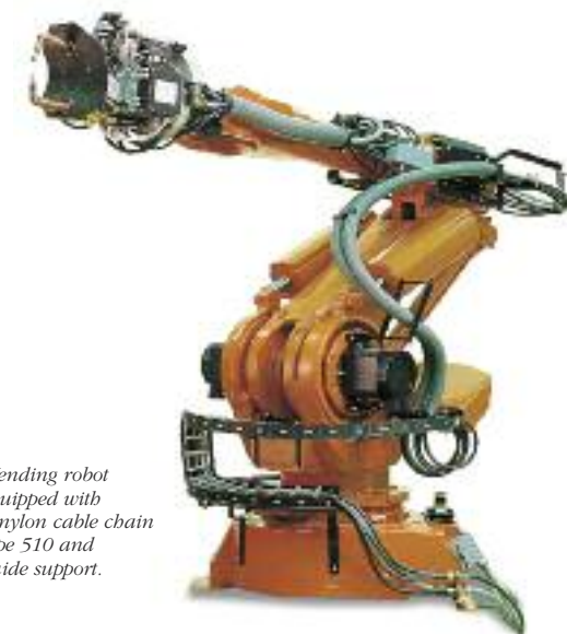
Circular nylon chains on welding robots.
