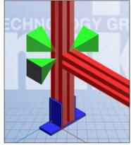
Floor mounting bracket rotated 90°
