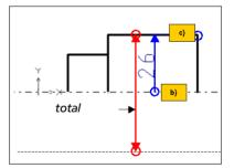
**Note:** Rotationally symmetrical points are dimensioned with the help of the "centerline dimension" function. Here the displayed dimension line describes half the measured distance only (therefore "half value"); however, the measurement value is the whole measured distance!
