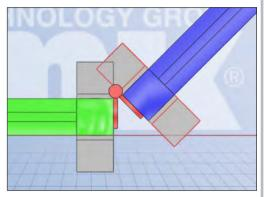
Step 3: Foot selection for blue-marked component can now be changed, e.g. from floor mounting brackets to end cap
