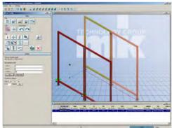
**Note:** Input point must be given or new part will be copied over existing part. This will not be visible on the screen and will cause unnecessary parts to be added to the final parts list.
