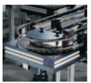
Rolling Curve 180° with adjustable side rails
