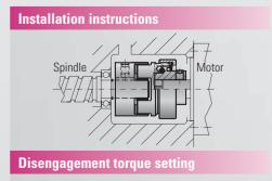
The ESL torque limiter is factory preset at the required disengagement torque and is not adjustable.
