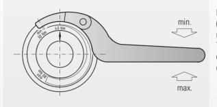
Miniature torque limiters (series 1.5-10) do not require a spanner wrench. These adjustment nuts can be turned with a bolt or a drift pin.
