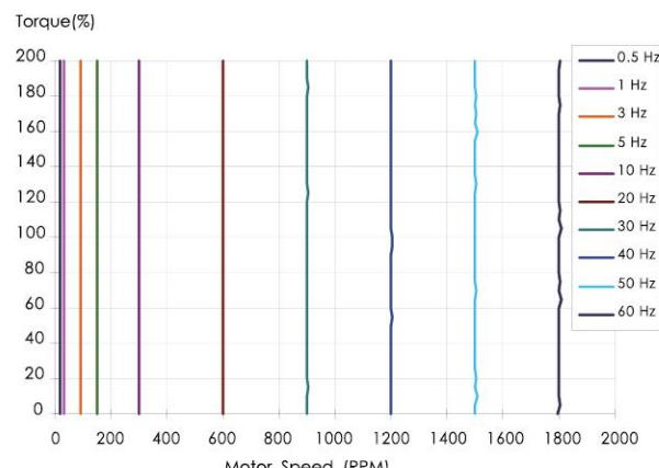
Sensor Vector Mode (SV) can output 200% holding torque.
