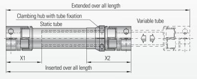
Inserted all over length = Extended over all length + Measurement ( X1 + X2 )
