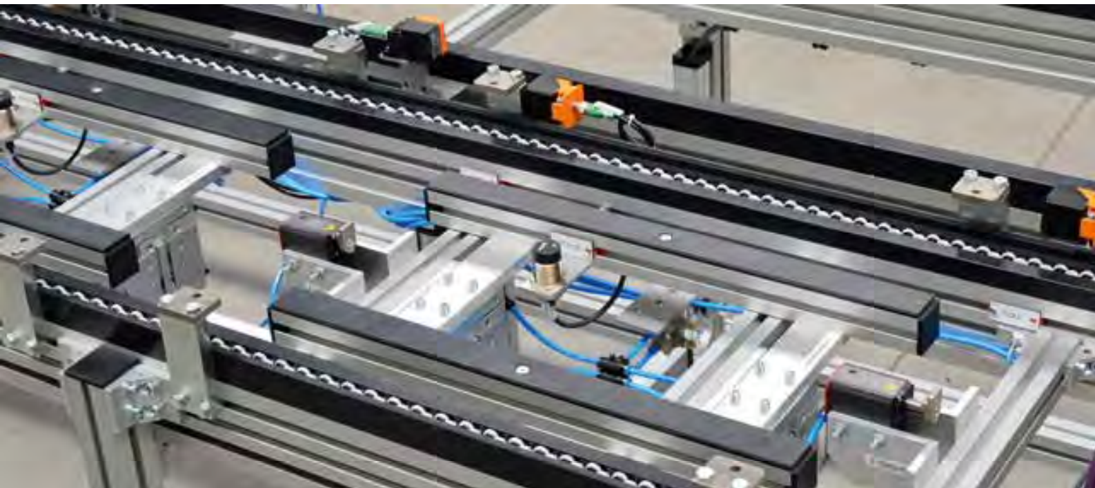
Robot unloading position with damped stops, pneumatic lifting with indexing from above, and RFID write/read module
