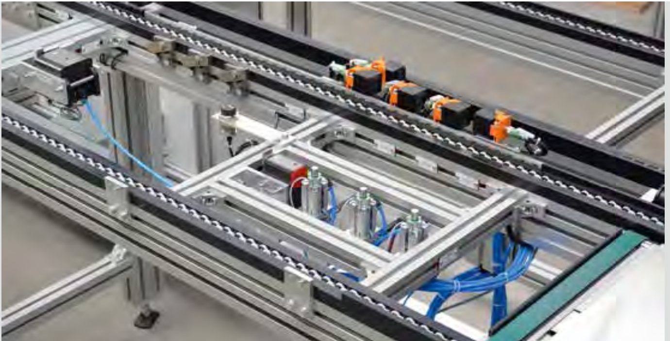
Station for 4 removal slots on a pallet with undamped stops and back stop. Accumulated pallets are separated upstream of the station in the process via damped stops on the buffer section.
