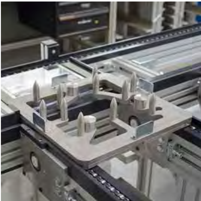
Customer-specific pallet, corrosion-resistant version for a cleaning system
