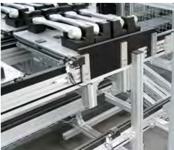
Confusion-proof parts receiving for left-hand and right-hand sided products
