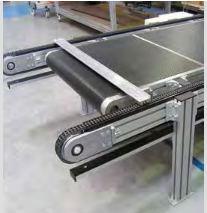
Combination of belt conveyor and chain conveyor with transverse rail for simulation of a floor obstruction
