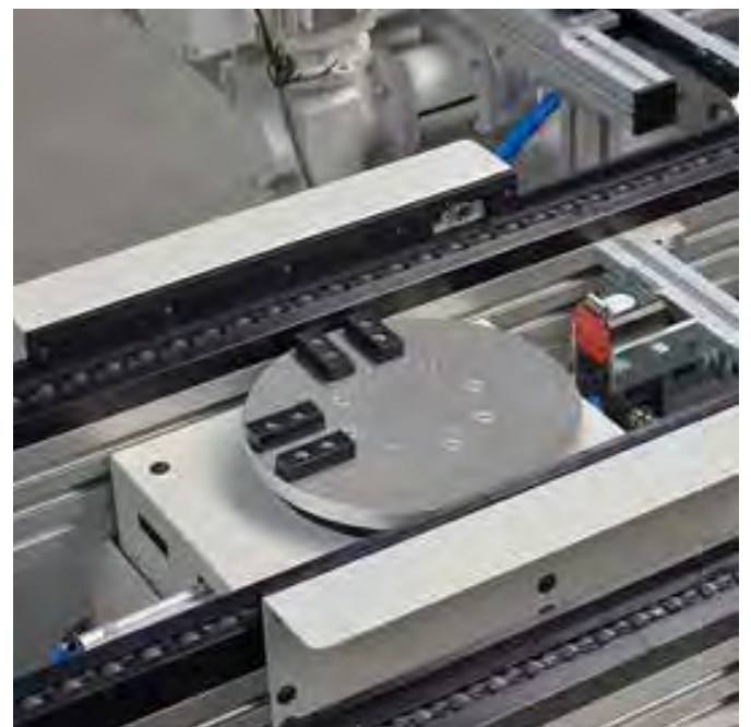
Fail-safe lift and turning station linking production cells in the automotive sector
