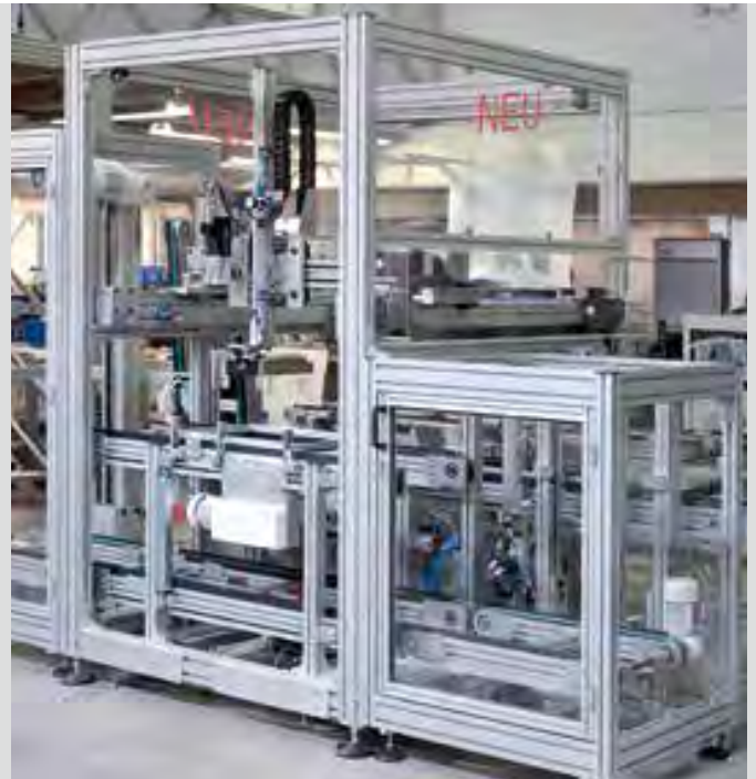
Pallet circulation system for various transport levels with 3-axis portal
