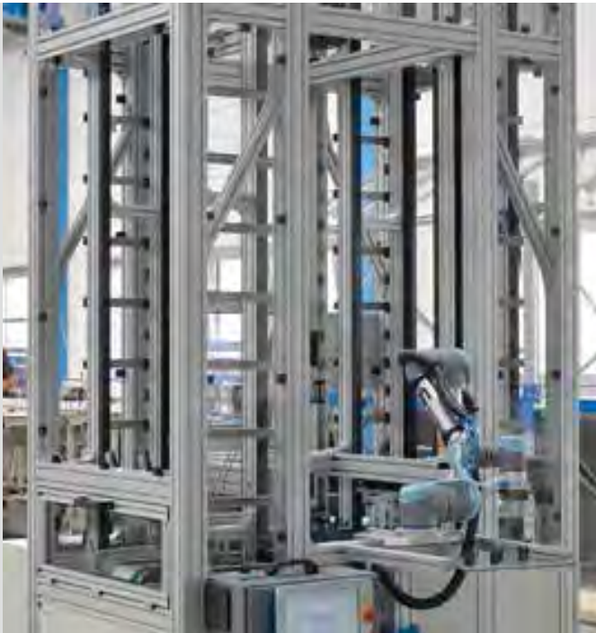
Lift and storage system for pallets with two chain conveyors running in opposite directions and pallet slots
