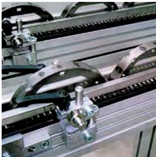
KTF-P 2010 with adjustable side rails and adjustable handles for frequently changing product widths
