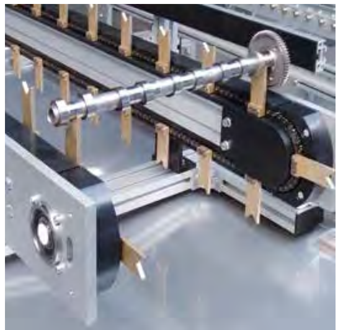
Chain conveyor KTF-P 2040 with prisms as pallets
