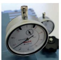
Control by comparator in 1/100 mm
