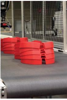
Low-noise fabric belt with fabric top cover for accumulation
