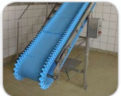
SuperDrive™ with sidewalls & special flights
