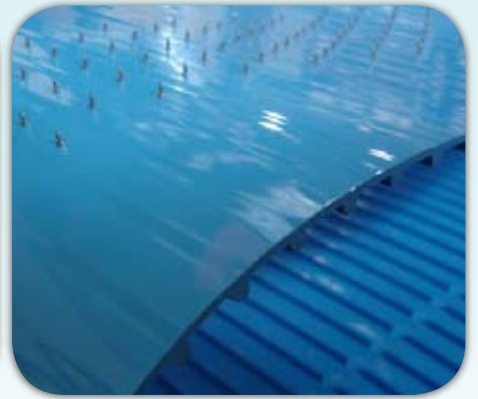
DualDrive Small Pulley with metal spikes
