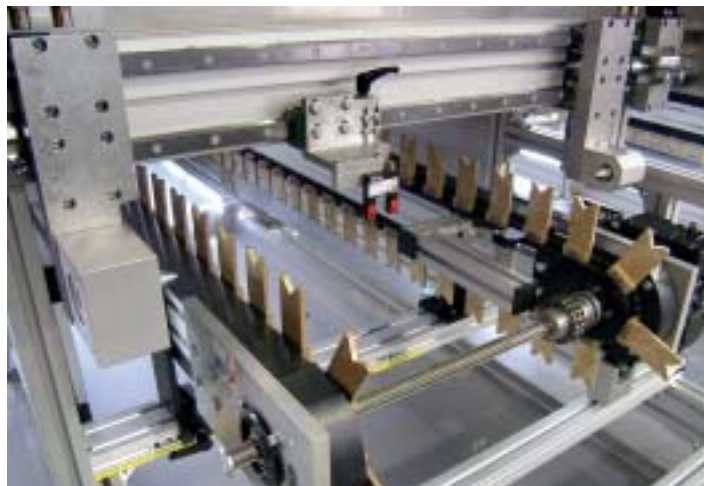
Linear assembly for manual lane width adjustment and clamping of the pneumatic centralizer and the electromotive turning unit
