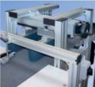
VST 2011 with digital display for width adjustment of the GUF-P 2000 AC side conveyor
