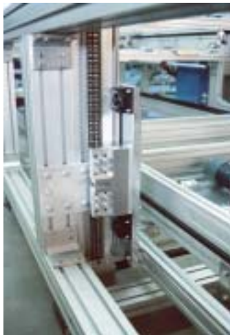
Linear module with duplex chain based on LZR 2005-38.44-30 as lift for pallet transport
