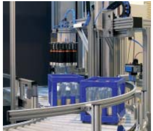
X-Z Axis combination with pneumatic drive and suction device for loading and unloading drink crates
