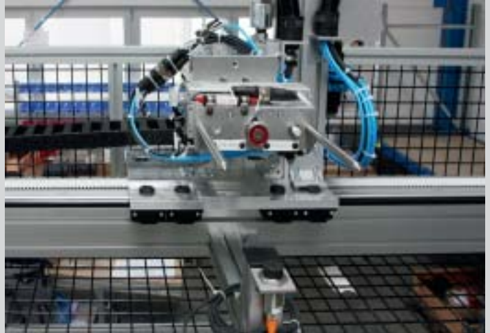
Horizontal slide carriage consisting of LZR 2005-38.44-30 linear module with fork-shaped gripper for transferring and unloading of workpiece baskets
