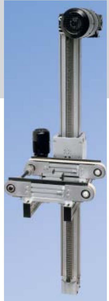
Linear Module with dual-carriage, asynchronous gearmotor, variable speed and triplex-chain as lift with timing belt conveyor
