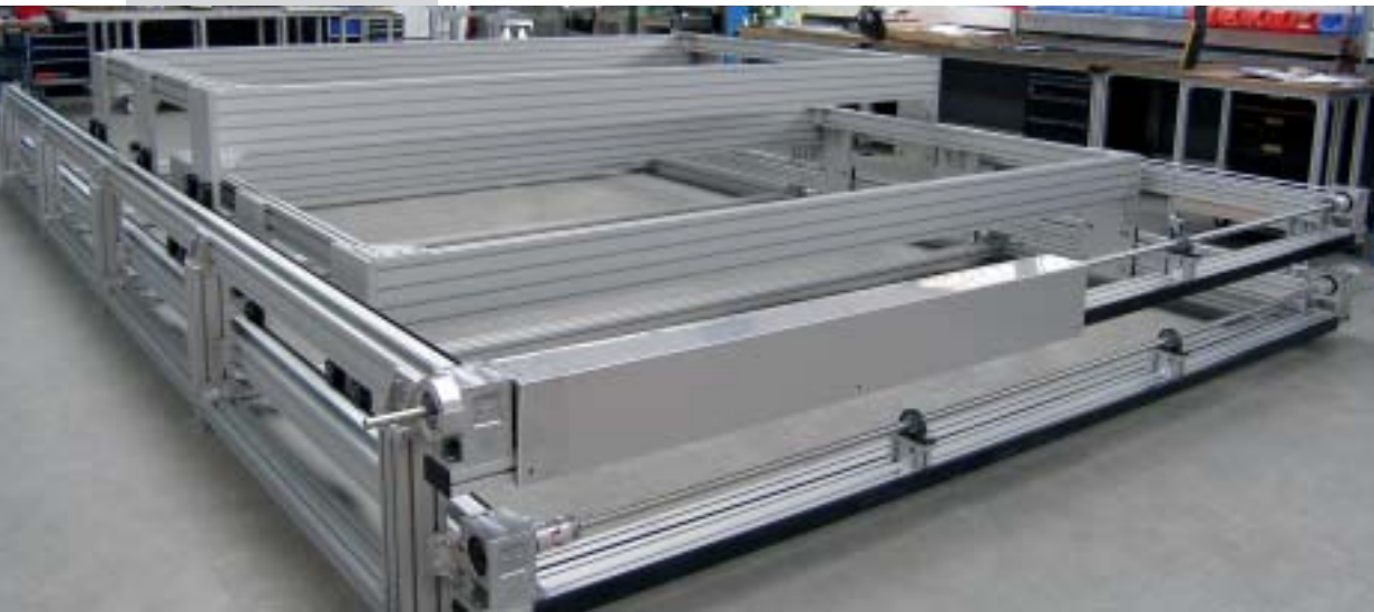
Double LZR 2011 -38.44-30 as changeable table for raw material plates. Product changes in two planes one above the other
