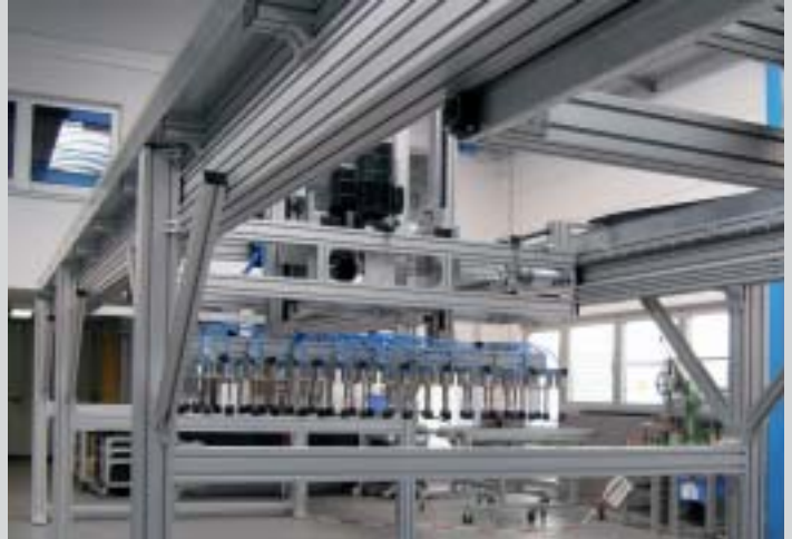
X-Z Gantry with vacuum gripper as handling and loading system of steel. Two independent loading systems on common X axis with guide rollers and riding rack drive
