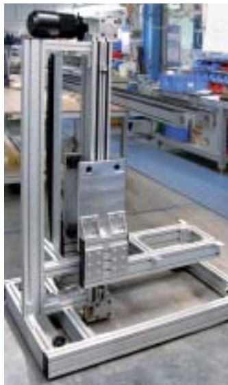
Lift with synchronous conveyor belt for transporting plastic bins. LZR 2005-38.44-30 linear module with two side carriages
