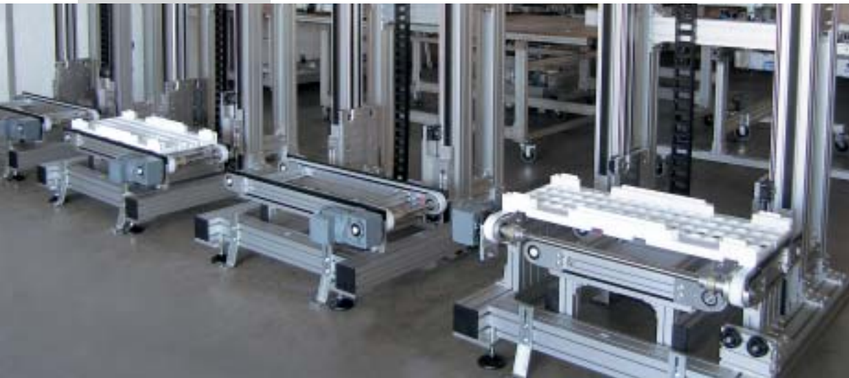
Lifts with 2-lane timing belt conveyor based on LZR 2005-38-44 with internally-arranged carriages
