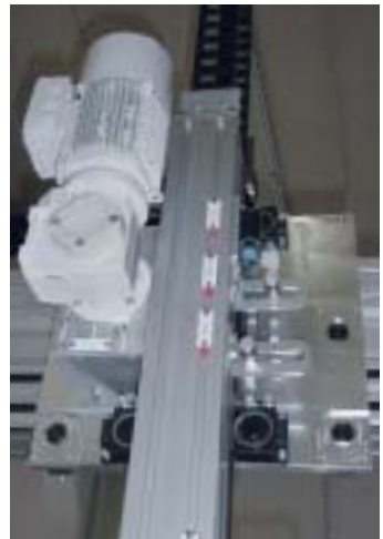
Two-axis application, Z axis with cross-carriage and Omega drive
