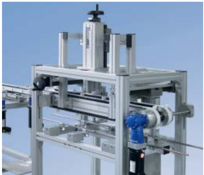
VST 2011 for manual adjustment of the conveyor height and double VST 2015 with timing belt coupling for width adjustment of the ZRF-P 2040.02 cycle conveyor
