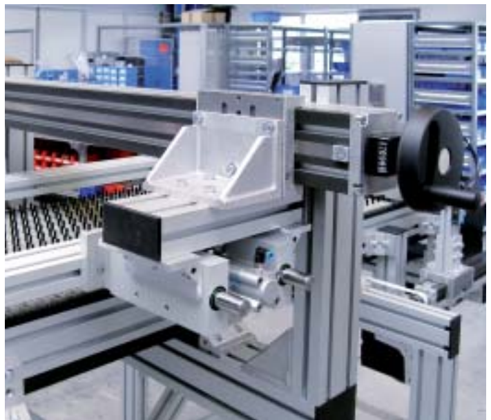
VST 2011 with digital display for width adjustment of the pneumatic centering unit on the modular belt conveyors
