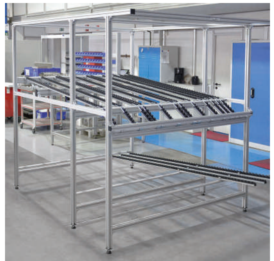
Kanban shelf with mini roller conveyors for material feed and empty crate return
