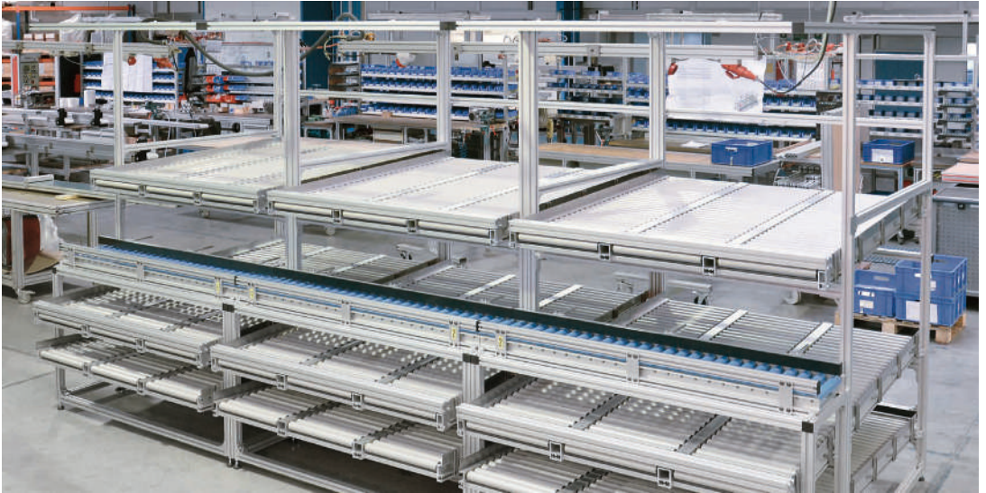
Kanban system workstation for manual removal and picking of products
