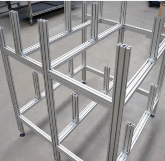
System frame built from mk 2025.02 profiles
