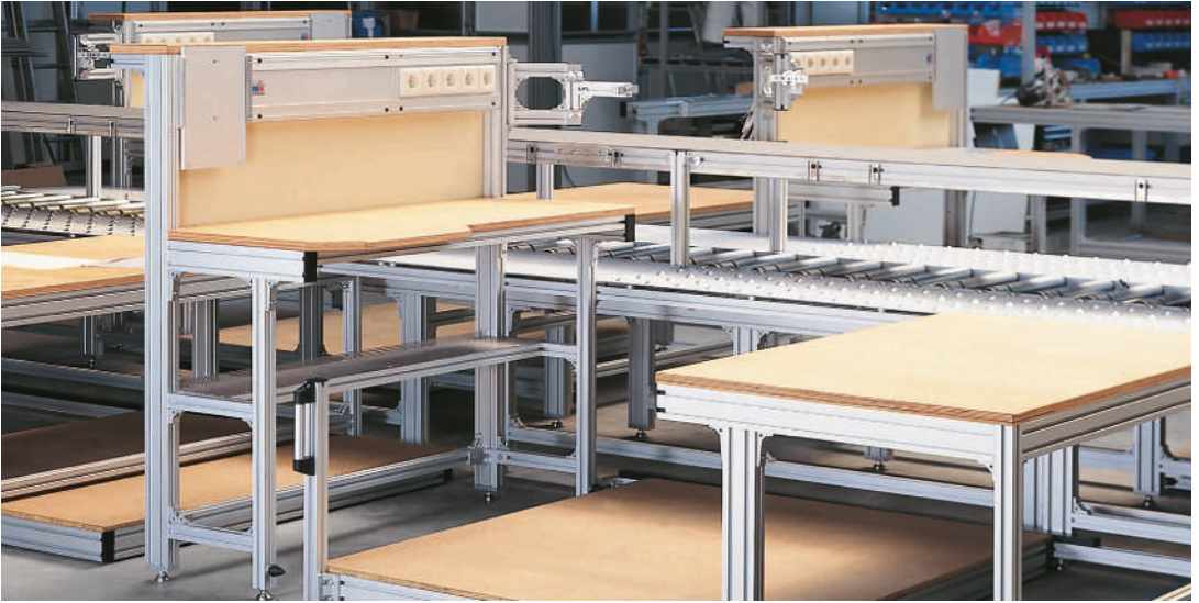
Interlinked industrial workstation with integrated electrical supply and driven roller conveyor
