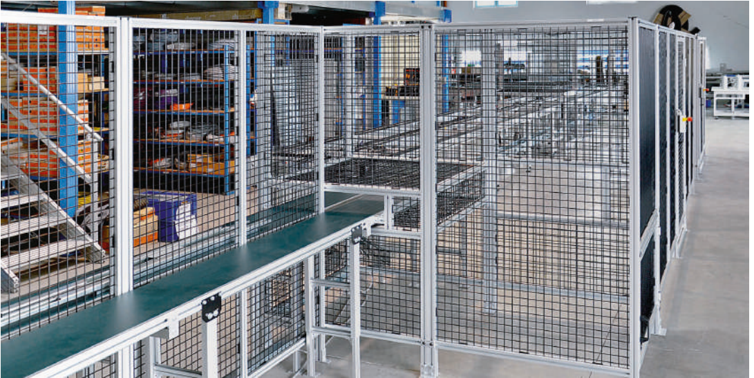
Guarding with welded grids (partition method) for tray transport system
