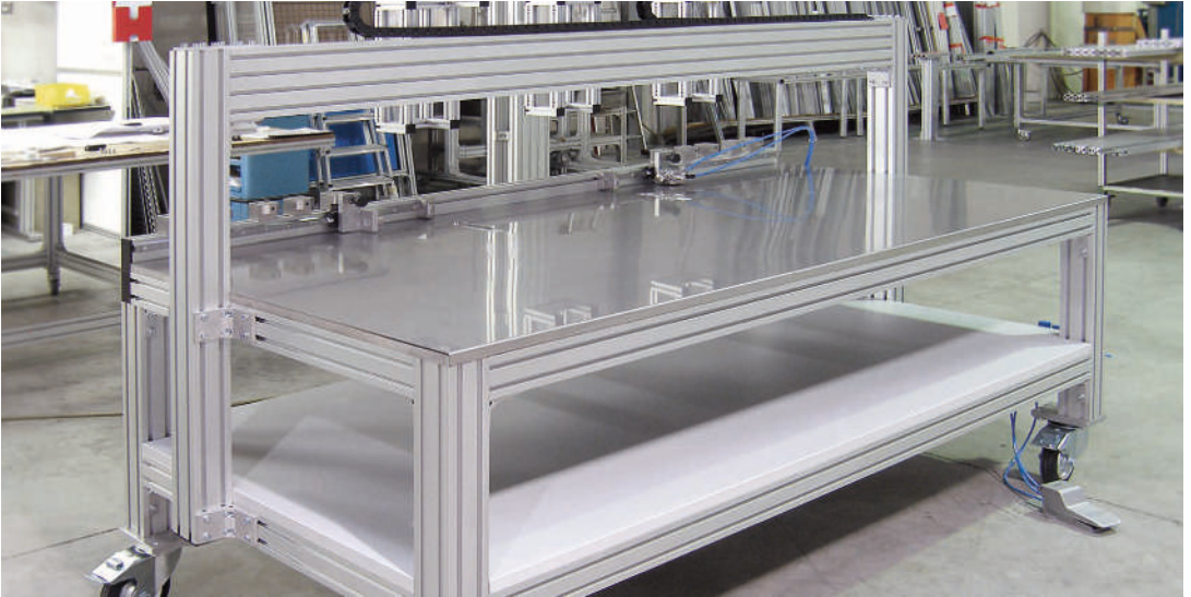
Custom assembly table with linear guide and pneumatic tensing device
