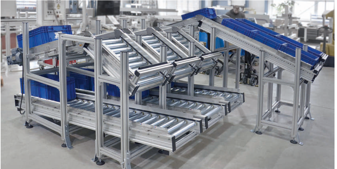
ESD-compliant loading and unloading station for feeding of small load carriers
