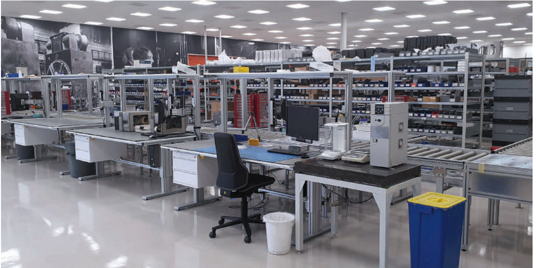
ESD-compliant assembly and test line with integrated conveying path for analysis units
