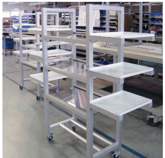
Material supply trolleys made from Series 40 cleanroom profiles with acrylic shelves
