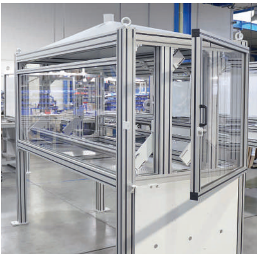
Charging unit for non-woven fabric production with maintenance door and extraction hood
