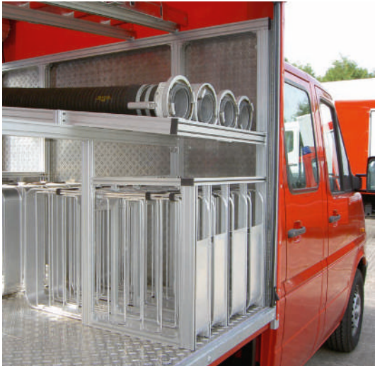
Fire engine interior built from Series 25 profiles
