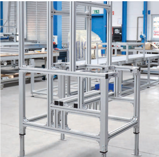
Machine frame made from Series 50 profiles
