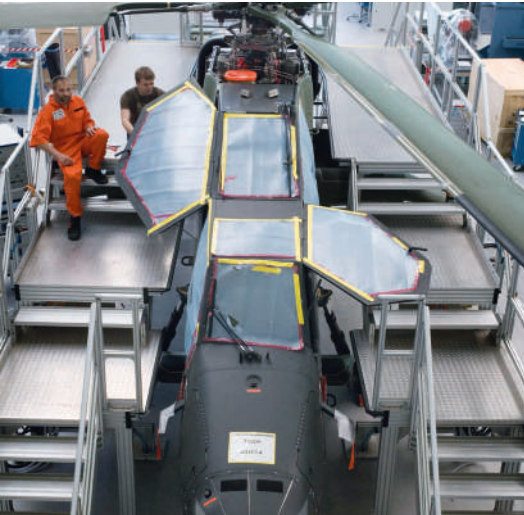
Mobile assembly platform for helicopters with different levels and multiple access points
