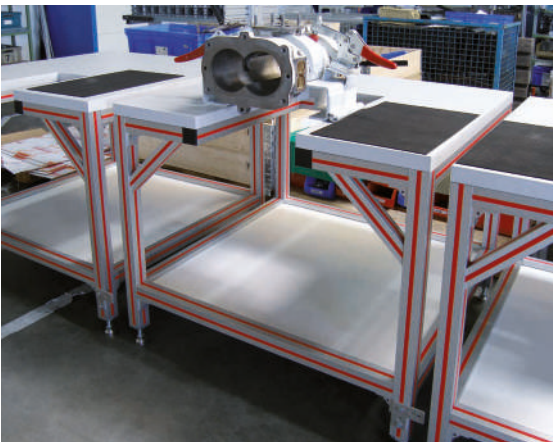
Assembly line for pumps built from Series 50 profiles with profile slots closed using red closure strips
