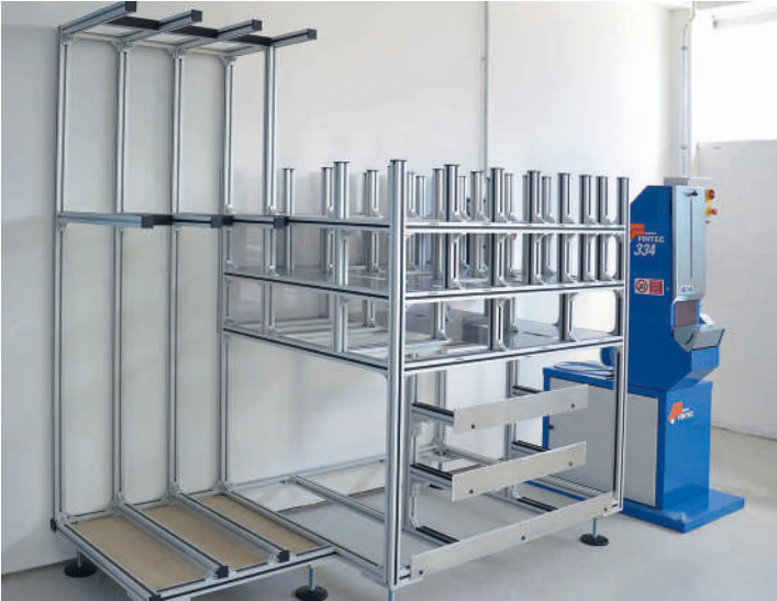
Custom material provision station for bar stock and individual parts
