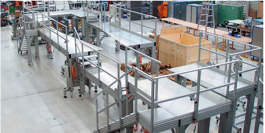
Free-standing assembly platform, 15 metres long, with high-load stairs for secure grip when carrying heavy loads
