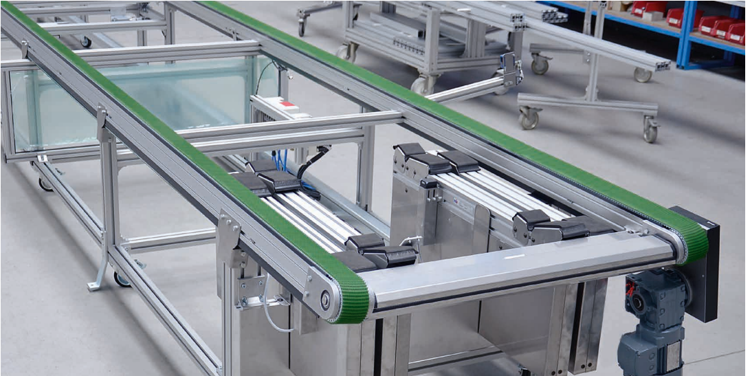
Dual-line timing belt conveyor ZRF-P 2040 with lines with 10° incline and lift at the outfeed
