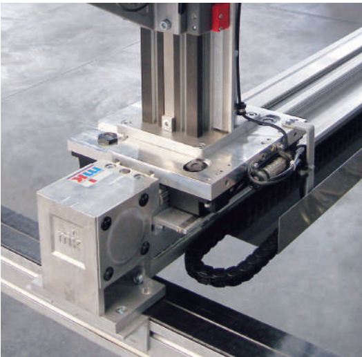
Linear module type LZR 2005-38.44-30 as a direct length measuring system with measuring head on the roller carriage
