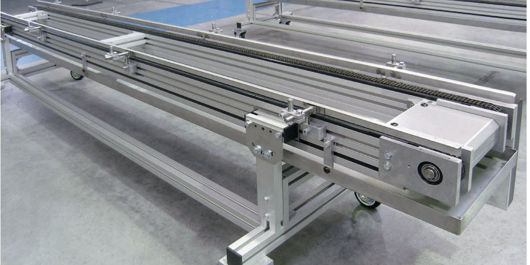
KTF-P 2010 with head drive AC with drip pan and movable support frame
