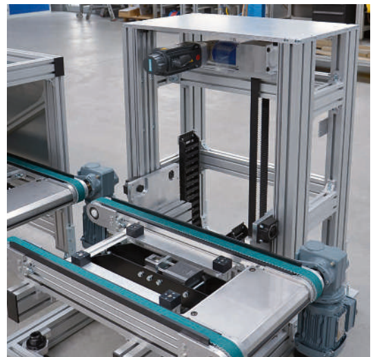
Short stroke lift based on PF-38.44 linear guide system
