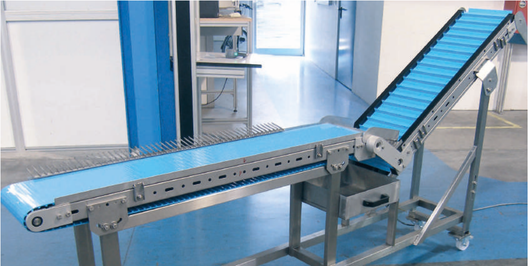
Combination of INOX belt conveyor and angled belt conveyor for transport of praline balls with granulate
