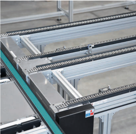
Dual-lane KTF-P 2010 with 80° C temperature resistance
