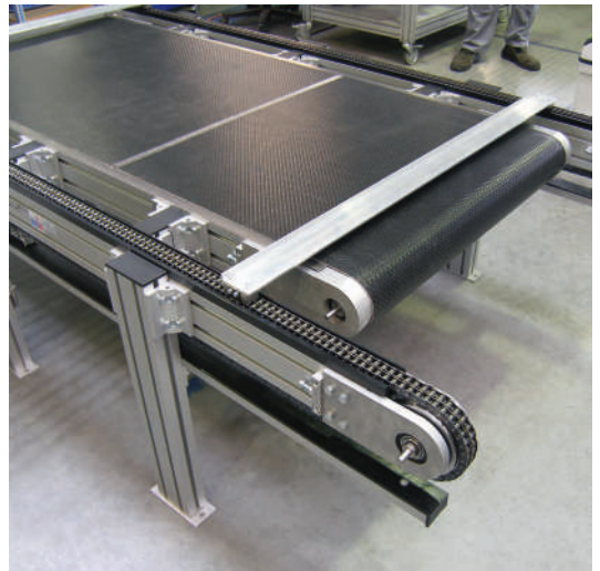
Belt conveyor combination of GUF-P 2004 with drum motor CA and dual line KTF-P 2004
