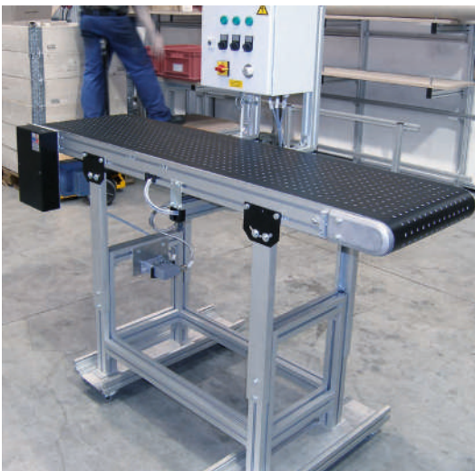
GUF-P 2041 with head drive AC and 90 watt fans in the conveyor frame, reglomat mounted on top of the conveyor frame
