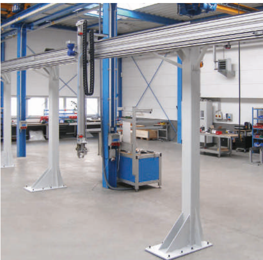
X-Z gantry with gripper for transferring crankshafts. X axis as LZR with support roller and timing belts, Z axis with timing belt Omega drive and fall arrest
