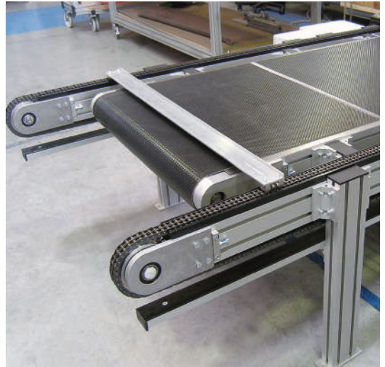
Combination of belt conveyor and chain conveyor with transverse rail for simulating a floor obstacle
