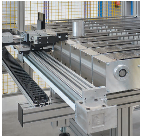
Linear axis from linear module LZR 2005-38.44-30 with movable gripping and transfer system
