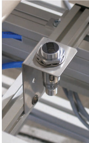
Initiator holder made from VA steel sheet
