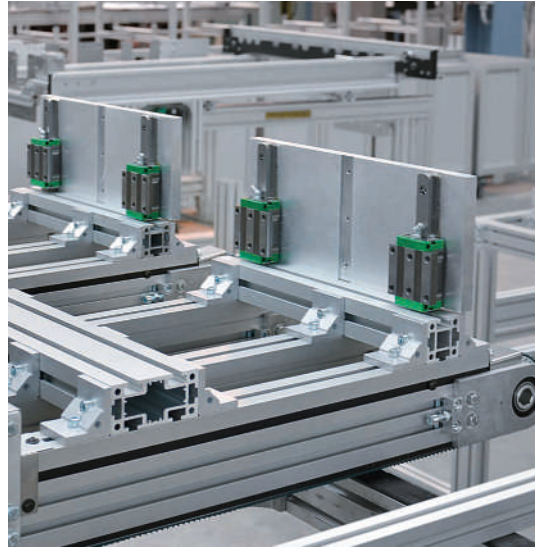
Lifting unit with KU 25 recirculating ball bearing guide and angle bracket
