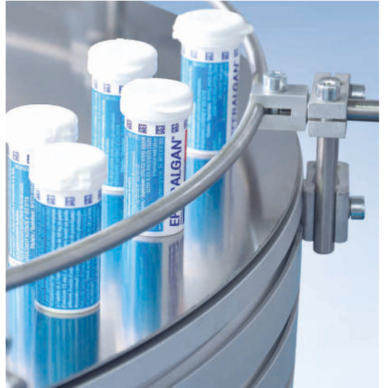
Rotary table DT-P 2040 with side rail, similar to SF01
