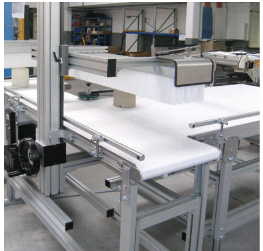
GUF-P 2000 with integrated adjusting unit (VST 2011) for height adjustment of the wiper brushes
