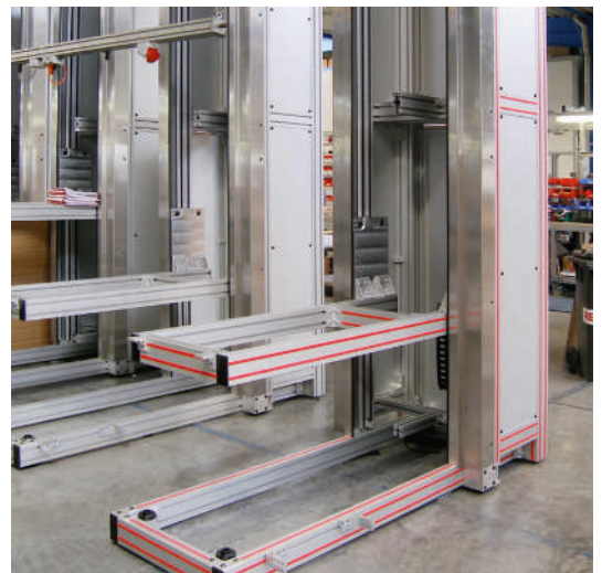
Dual linear module type LZR 2005-38.44-30 with cantilever for conveyor as a lifting unit
