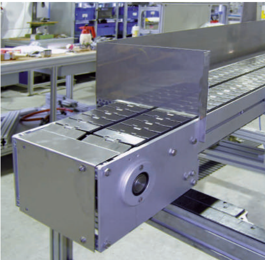
Double-line flat top chain conveyor with one motor
