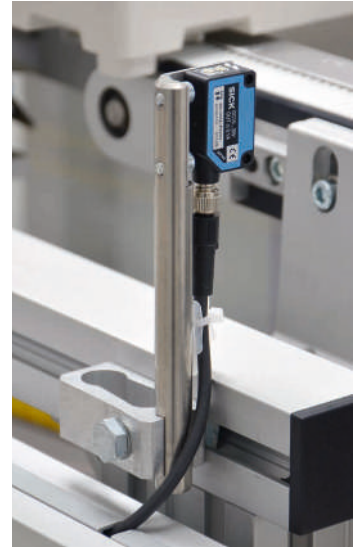
Photoelectric sensor with adjustable holder
