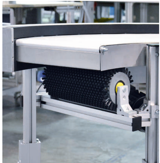
Wiper brush, rotating, mounted at the end of the conveyor
