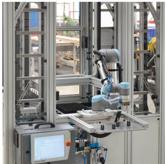
Production cell with patenoster storage for infed and discharged parts
