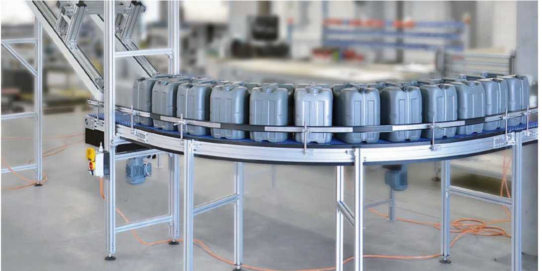
KMF-P 2040 as an infeed for empty canisters
