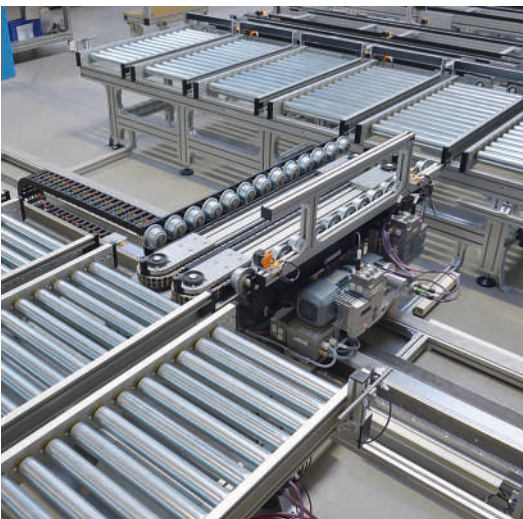
RBT-P 2255 roller conveyor as a storage conveyor with central loading and unloading tasks
