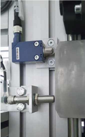
Sensors for deceleration and stopping
