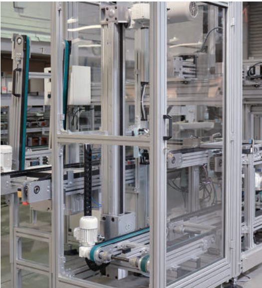
Electrically driven lift in "stand-alone" frame with guarding
