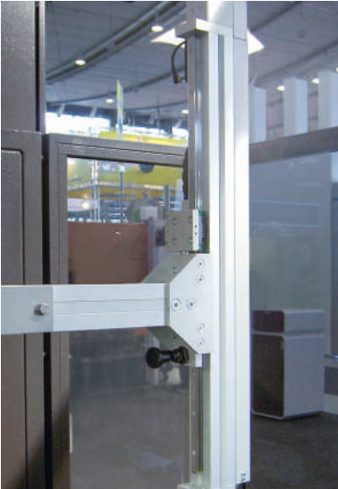
Electromotive VST 2015 with recirculating ball bearing guide
