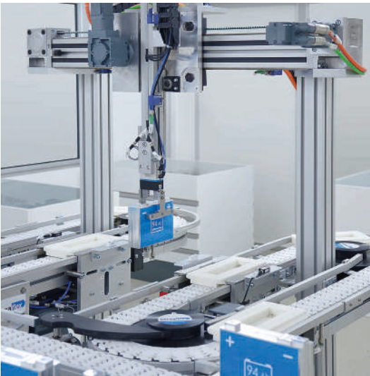
Two-axis gantry with servomotors and custom gripper in combination with Versaflex flat top chain conveyor
