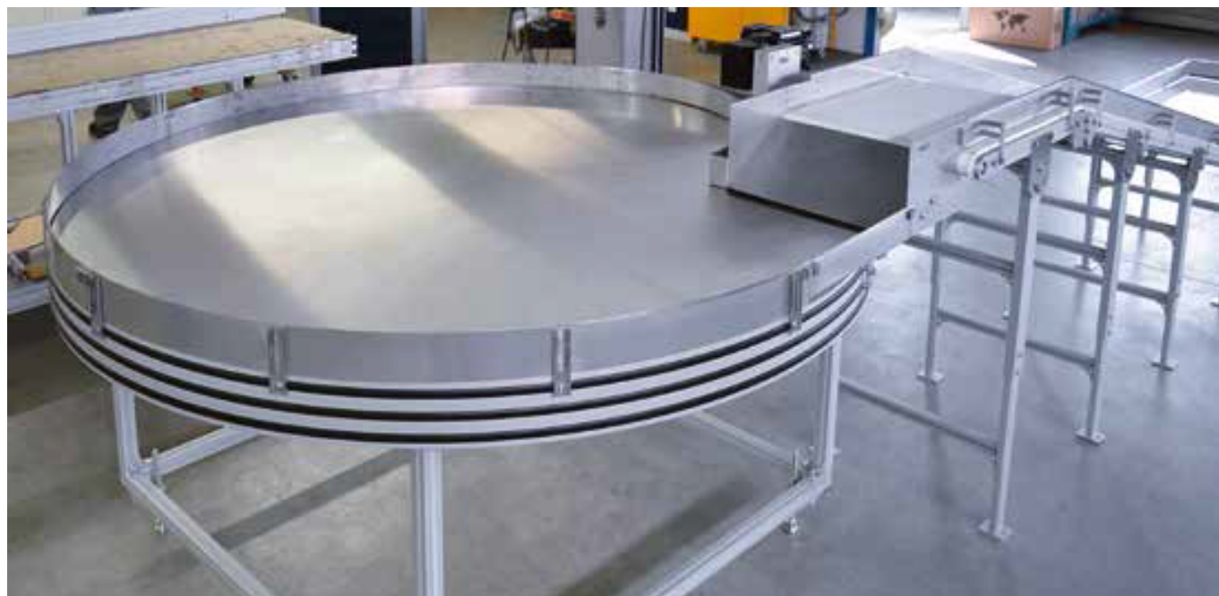
Turntable "light" with timing belt drive (ø 2000 mm), applications in the pharmaceutical industry
