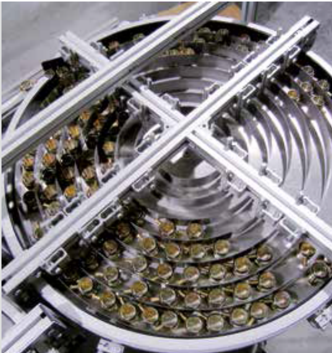
DTZ-P 2040 swivel table with timing belt drive
