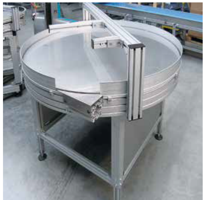
Turntable with direct drive, perimeter stainless steel plate and single-strand discharge
