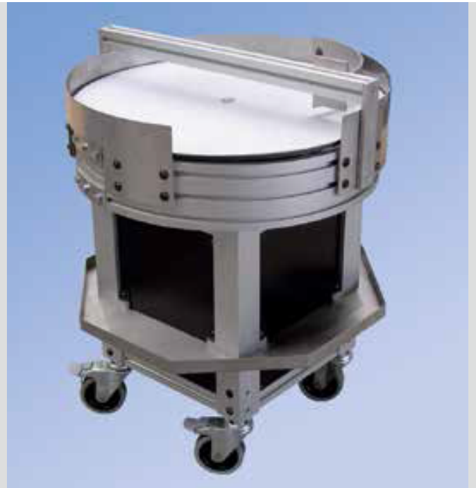
Turntable with direct drive, perimeter stainless steel plate and leader gage plate in the feed area
