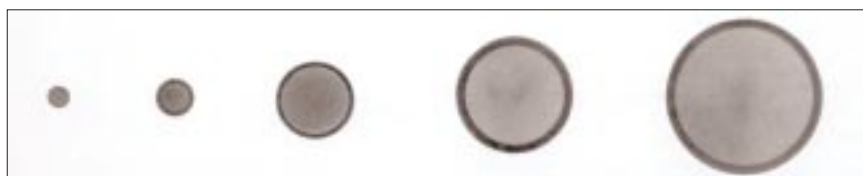
Pictures showing controlled hardened zone
