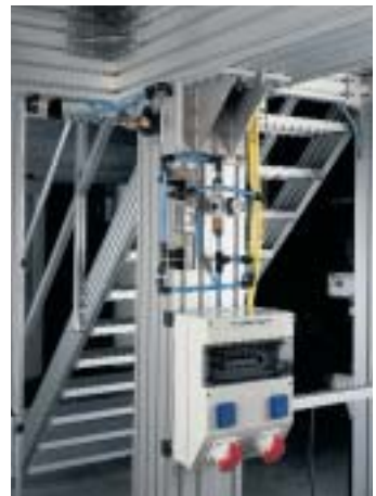
The mk profiles provide space for electric, pneumatic and hydraulic supply lines
