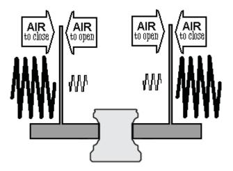
Using a 5/2 ways valve, the force produced by the spring is complemented by the one produced by air pressure; with this variation the clamping force is increased by 2.5 times.
