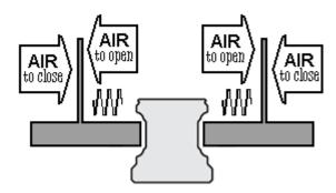
The operating principle is the same as normally open, except for the release phase, which is assisted by air. The vent is replaced by connecting a second air duct (using a 5/2 ways valve).
