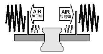
The locking element closes by means of a spring, and air pressure is used in order to open.
