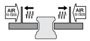
The locking element leaves the guide free to slide. Locking is done by forcing air into the element to activate the closing. The system is unlocked when the air pressure is removed.
