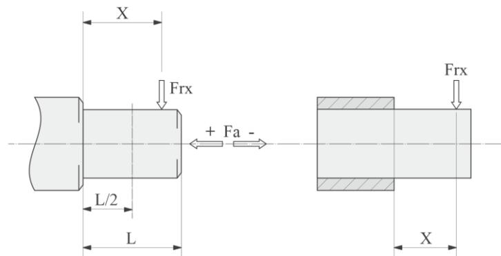
Allowable overhung and axial loads on the output shaft  $F_{h2} \cdot n^2 \cdot h = 100000$
